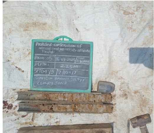
fig-9 Recording SPT-N Value
